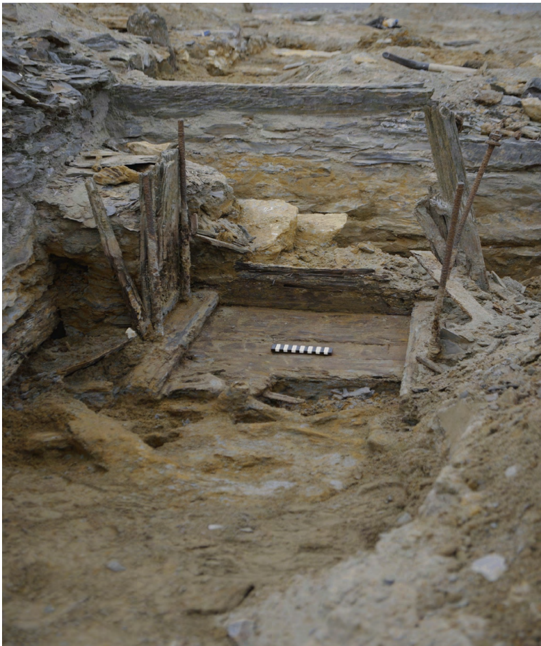
No. 8 [above, to N: left, detail to E]. Excavation showed that this buddle had been dismantled and removed sometime after Moissenet's plan was drawn, and had been replaced by jiggers, of which only one remains: this was also excavated.
